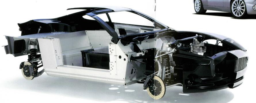
The architecture of the Vanquish is made of extruded aluminium sections bonded and riveted around a carbon-fibre central transmission tunnel.
