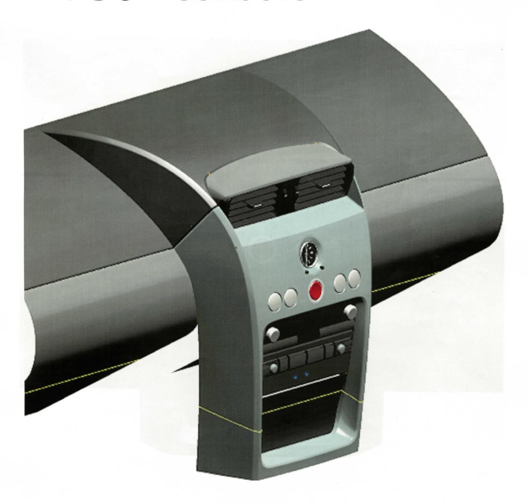
X100 registers with redesigned face incorporating centre thumb wheels re-aligned switches altered surface around clock chamferred console
