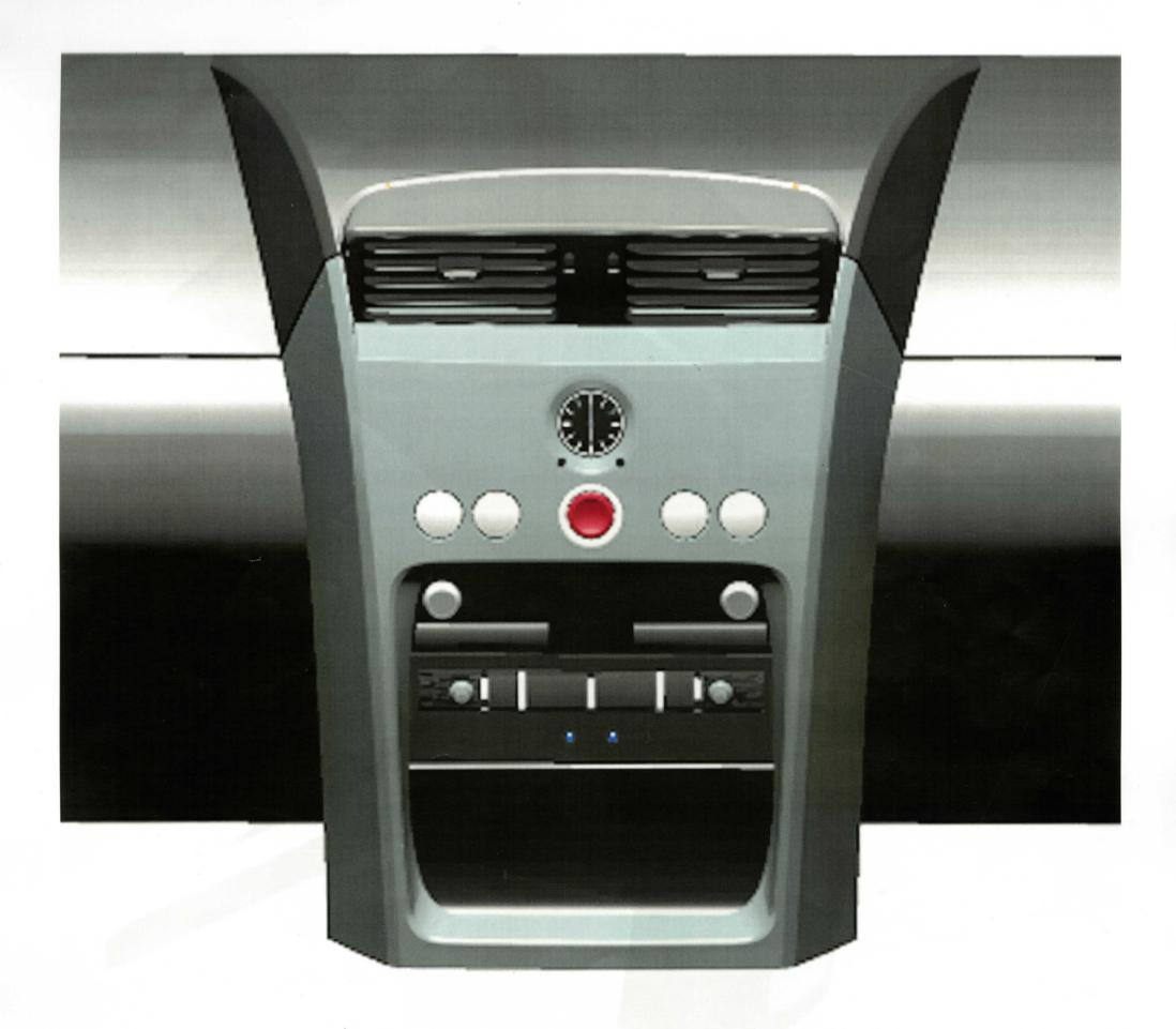
X100 registers with redesigned face incorporating centre thumb wheels re-aligned switches altered surface around clock chamferred console
