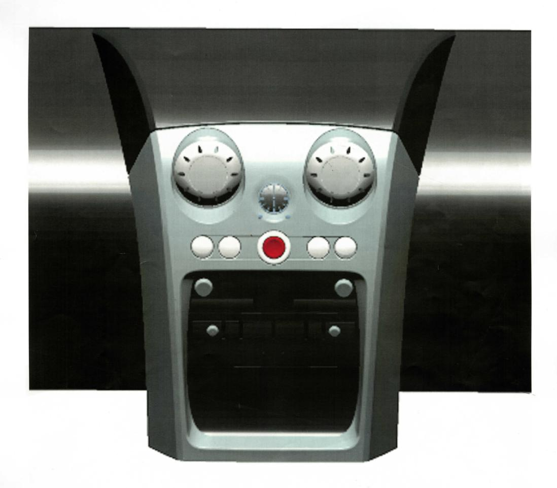
90mm vents positioned below shut line 50% into the surface re-aligned switches altered surface around clock chamferred console
