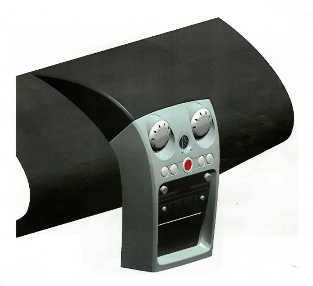
90mm vents positioned below shut line 50% into the surface re-aligned switches altered surface around clock chamferred console
