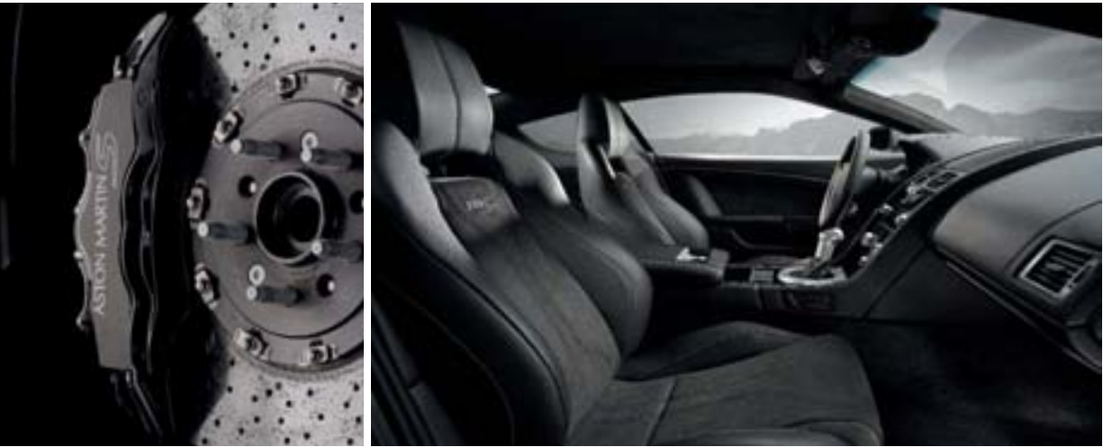
FAR LEFT: For the first time on a road-going Aston Martin, Carbon Ceramic Matrix (CCM) brakes are employed, resulting in shorter stopping distances with excellent resistance to fade in even the most demanding driving conditions.
