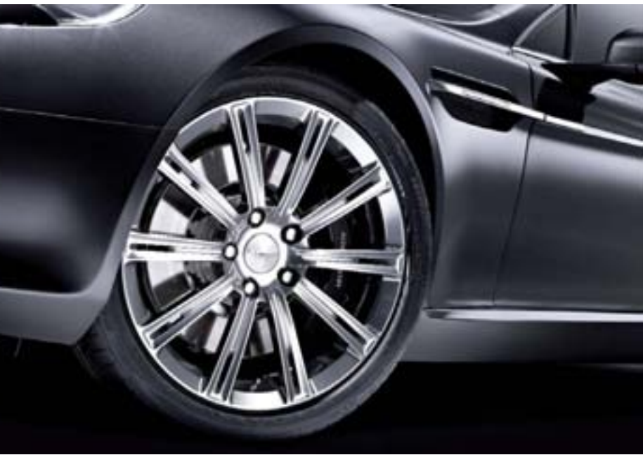
Rapide Luxe's exclusive 20" 20-spoke wheels have a high-clarity polish achieved through an intensive process lasting 90 minutes per wheel. A series of seven machines polish the alloy to a fine finish using ceramic spheres.
