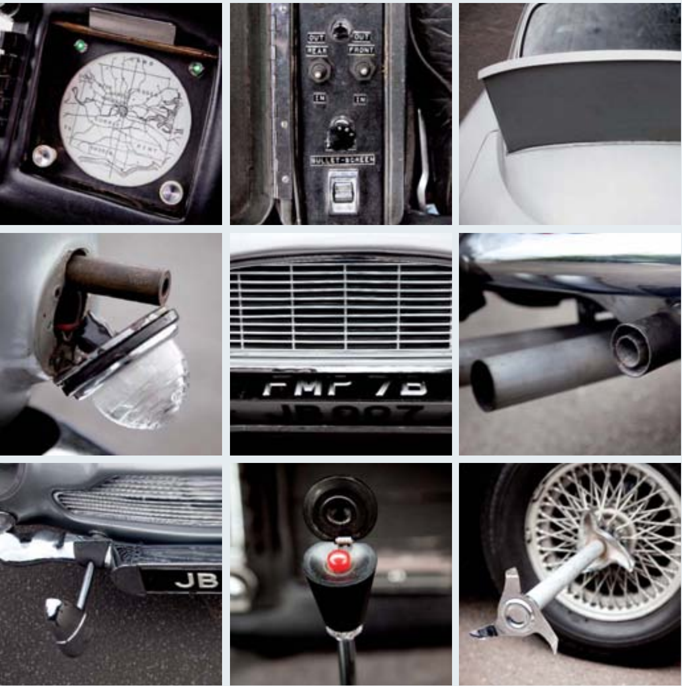
ABOVE: For Goldfinger and Thunderball , four DB5s were fitted with ‘all the usual refinements’, as Q described them. The pop-out machine guns, tyre shredders, bullet-proof screen, revolving number plates and ejector seat were designed by Oscar-winning special effects guru John Stears, who went on to work on Star Wars .
