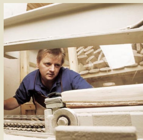
ABOVE: Gary Sandford of Cricket First Choice, pressing the willow blade with a weighted hydraulic roller.
